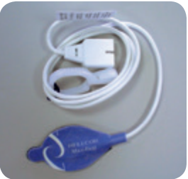
MAXFAST-1 Reflectance Sensor Can be applied to the tail (wrap included), designed for head and neck surgery or dental procedures.
