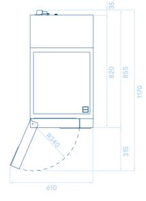
Sterilization chamber sizes (mm)
